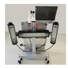
To capture data of light and thermal waves passing into and out of the material, we use a high-performance IR thermographic camera capable of capturing temperature modulations from the entire observed body surface at once. On the basis of taken images, the patented algorithm of ThetaScan software, performs amplitude and phase processing of the temperature path. Using the "Fourier Analysis" algorithm, each pixel is processed individually for each recorded image.
